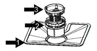
The filter system consists of a coarse filter, a flat (Main filter) and a micro filter (fine filter).
